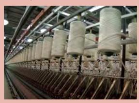
Spinning twists the fibres into a continuous yarn
